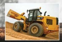
Tire pressure monitoring and auto-lube systems from third parties have been around for quite a while. However, manufacturers have not really had solutions like these in a fully integrated format before, especially when it comes to small wheel loaders. Caterpillar, on the other hand, has been working hard to develop its own, in-house solutions.
