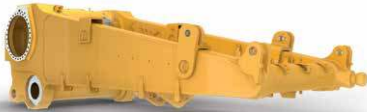
Improved case and frame to increase fatigue life
